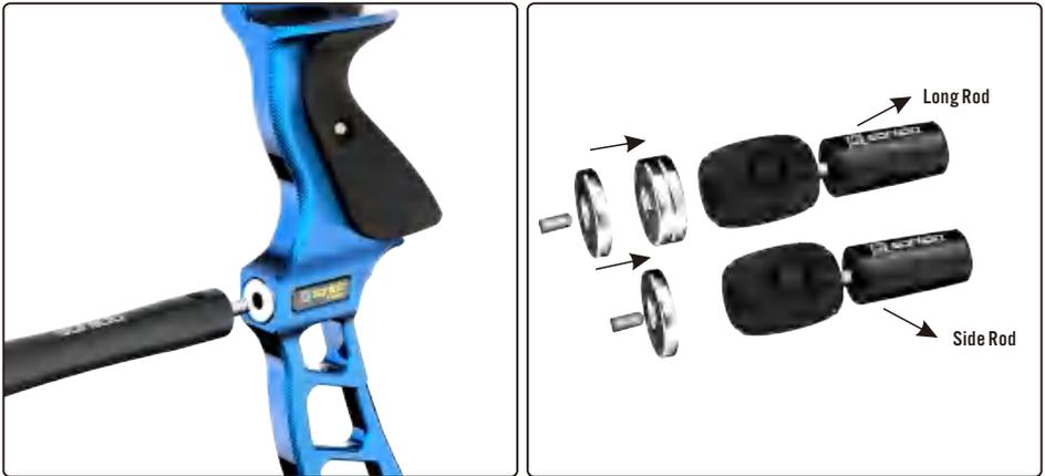
First tighten and fix the V - bar and the extender together, then screw the 5/16-24UNF screw at the other end of the side rod into the quick connector, align it with the round hole on the V bar, insert and tighten it to ensure firmness. The 5/16-24UNF screw at the other end of the long rod shall be directly tightened with the screw hole on the connector to ensure firmness.
